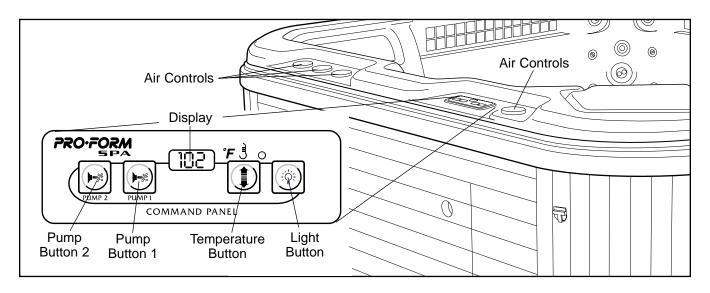
Refer to the diagram above. The function of each control is explained below:
